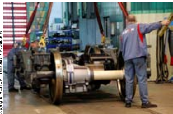
The AGV™'s power bogies are built at Alstom's Le Creusot site
