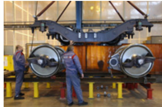
The AGV's powered bogie formed part of the traction system for the train that broke the world rail speed record by travelling at more than 574.8 km/h on 3 April 2007.
